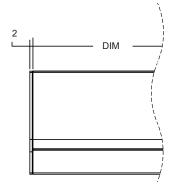
Note:- length dimensions are not including end caps. (2mm per cap will be added to total length)
